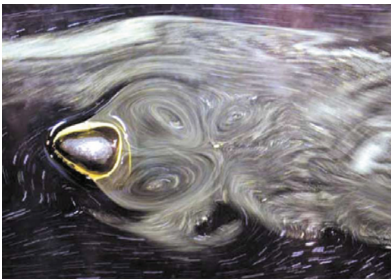
Fig.4. Twin vortex (left) and Kármán vortex (right) behind a rock of river (Surface floating method using pollen of pine tree)
