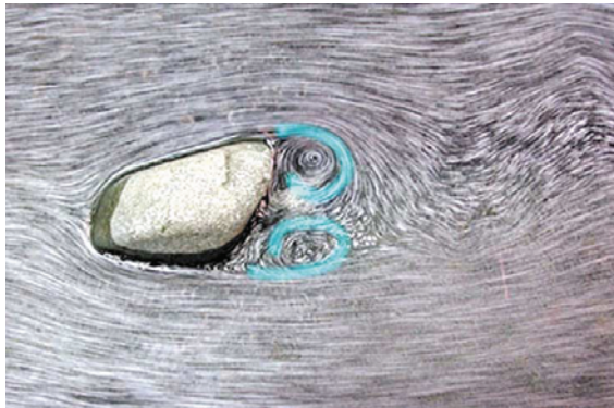
Fig.3. Twin vortex (left) and Kármán vortex (right) behind a rock of river (Surface floating method using pollen of cedar tree and aluminum power)
